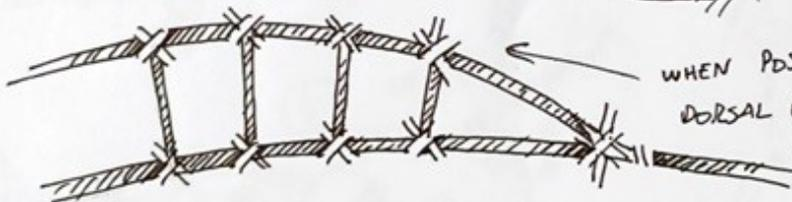
WHEN POSITIONING STRUTS TO MAKE DORSAL FIN, PUSH, SLIGHTLY, AGAINST SUPERSTRUCTURE TO MAINTAIN TENSION
